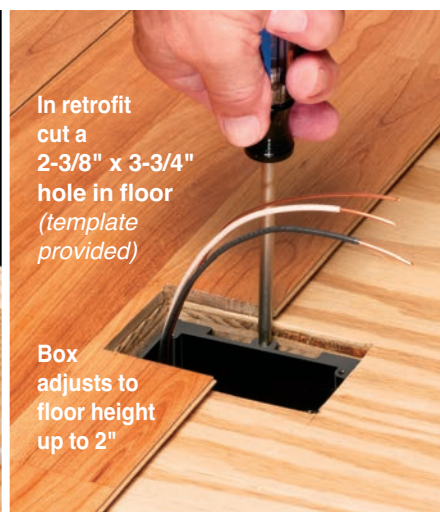
3 Adjust box height and install bracket
