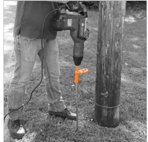
Tool locks into hammer drill
