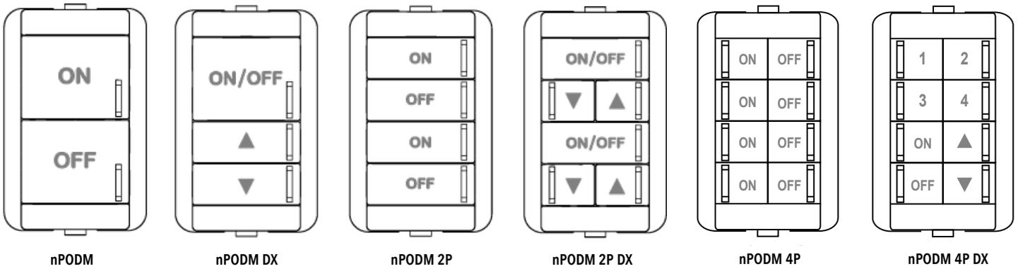
Dynamic wallpod options feature custom button names when pairing with Acuity Brands nTUNE(TM) fixtures. Reference fixture cut sheets for additional details.
