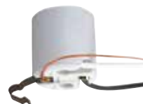
*22372 Porcelain Snap-In Socket Medium Base 9" Wire Leads Fits ¾" x 1/4" Hole 18 Gauge, 105° Leads 660 Watts Max., 250 Volts Height - 2"
