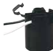
*22217 1 ½" Snap-in Socket 9" Wire Leads Medium Base Fits ¾" x 1/4" Hole 18 Gauge 105° Leads 660 Watts Max., 250 Volts Height - 1½"
