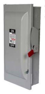
Siemens Low Voltage Circuit Protection General Duty Safety Switches. Type: ENCLOSED, SAFETY SWITCH Std: UL V. Rating: 240V A. Rating: 100A Wattage: 3W No. Of Poles: 3P F. Rating: 60Hz Action: SINGLE THROW Material: STEEL Enclosure: TYPE 1. 2-3 point mounting holes. O. Cycles: 10000 O. Temperature: (-20F-120F) AMBIENT TEMPERATURE Environmental Conditions: INDOOR
