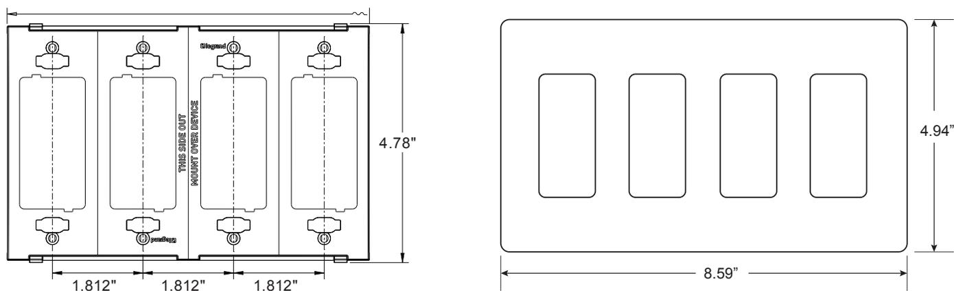
Align subplate over NEMA 26 sized electrical devices and receptacles. Affix subplate with included screws to electrical wall box. Secure tightly, but avoid over torquing screws. Snap on radiant screwless wall plate to subplate.
