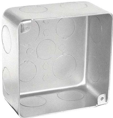
Chicago plenum, 2-1/8" deep, 4" square drawn boxes with air tight (8) 3/4" side knockouts and (3) 1/2" & (2) 3/4" bottom knockouts are installed in air plenum walls or ceilings spaces for lighting fixtures, switches, receptacles or other outlet devices. Square boxes are used to bring power to a number of electrical devices where multiple conductor runs are split in two or more directions.
