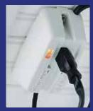
The Roof Sentry RS2 unit automatically controls operation of ADKS electric roof de-icing cables. It measures both temperature and moisture to turn the system on or off in response to changing weather conditions.
