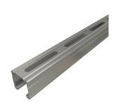
14 Gauge Slotted Strut Channel P1100SL has long slots on the back side for use with 3/8" threaded rod and fasteners. These slots can eliminate the need for field drilling and allow adjustability when installing. The slots are 3" long with 1" spacing.
