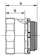
Fittings are Furnished with Insulated Throat Bushing Eliminates Anti-Short Bushings or Red Heads
