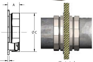
Illustrated Thru Wall Application 2 Braces on Conduit
