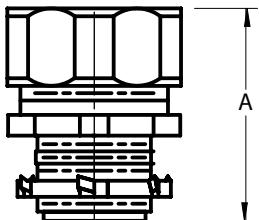
Connector Furnished with a Steel Locknut
