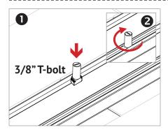
**PLACE T-BOLT INTO RAIL & SECURE BOLT:** Insert 3/8" T-bolt into rail at L-foot locations. Apply Anti-Seize to bolt. Rotate T-bolt into position.
