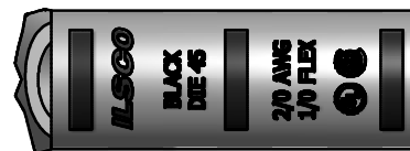
DETAIL A, SCALE 1.8 : 1 TOP INK MARKING INK COLOR: BLACK PER SPEC #: F921
