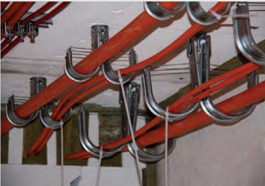
J-Hooks and cables in fire chamber before fire test
