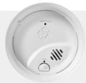
SMI105-AC Hardwired ion smoke alarm, 120V with sealed 10-year lithium backup, 85 dB horn, interconnectable up to 18 units
